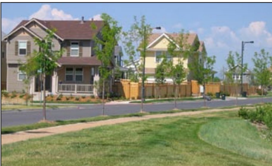
A gravel trail replaces a concrete sidewalk and promotes infiltration.
